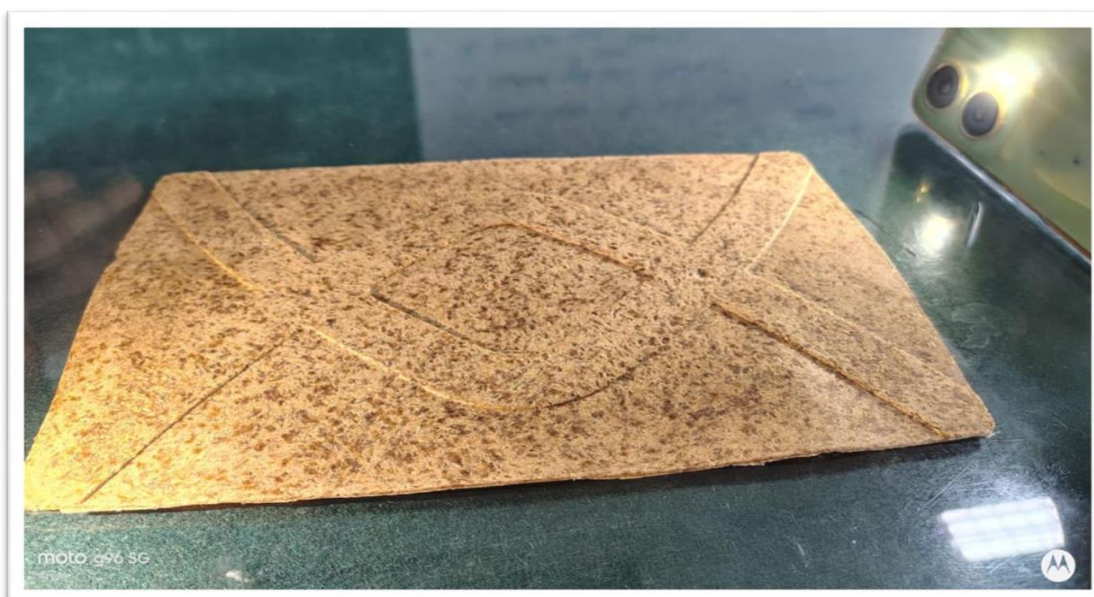
Fig 1. Mycelium based MycoVogue Bio-leather
